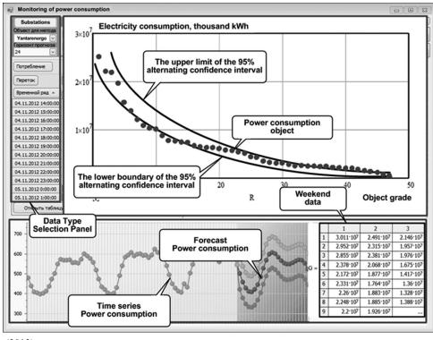
Figure 5: Desktop for calculating energy saving potential
